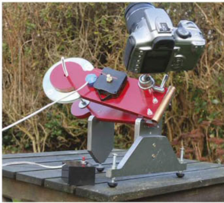
▲ The finished mount allows you to take longer-exposure photos before stars begin to trail
